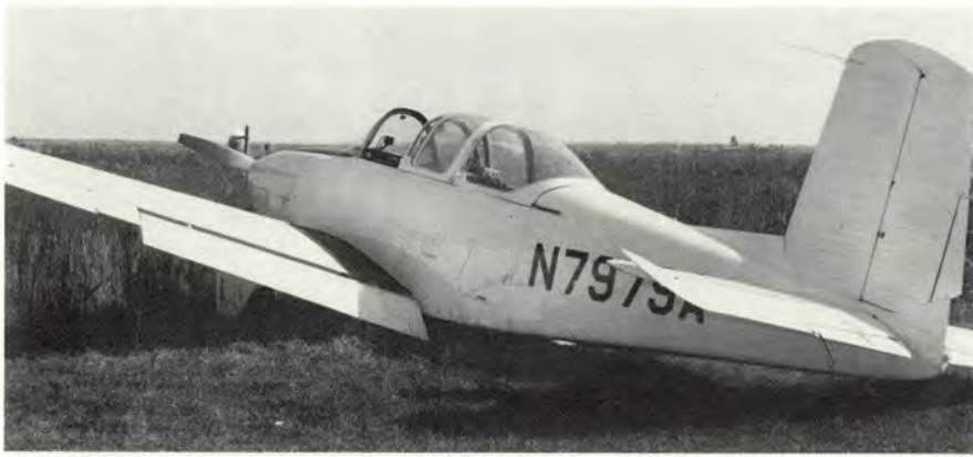
2. 1969—T-34 right main gear collapsed during landing. Aircraft swerved off.
