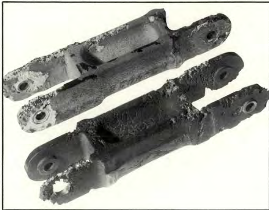
F-105 Flight Control Stick Link Rod Corrosion PN 79F340012-1
